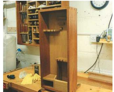
▲ Pic.23 ...to finish the saw cabinet, which is awaiting the French cleats
